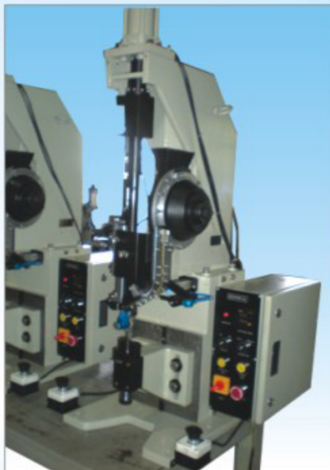
Auto Feed Riveting Machine for Tubular Rivets
