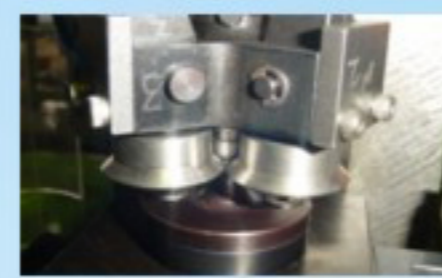
Auto Feed Riveting Machine for Tubular Rivets
