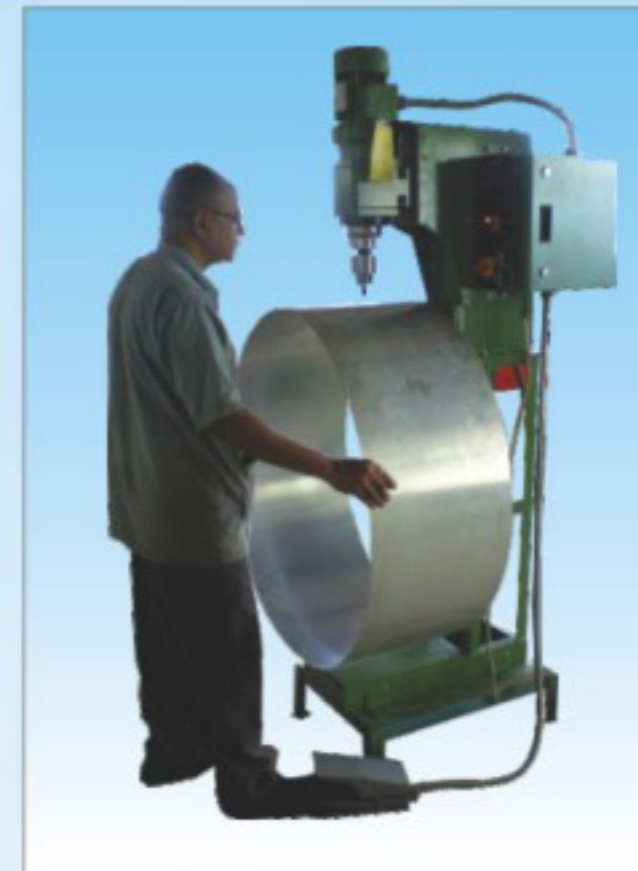
Riveting Machine for Big size Circular Job
