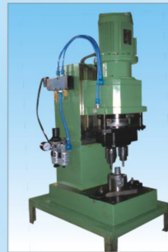
Riveting Machine with Twin Spindle Attachment & Component Locating Fixture
