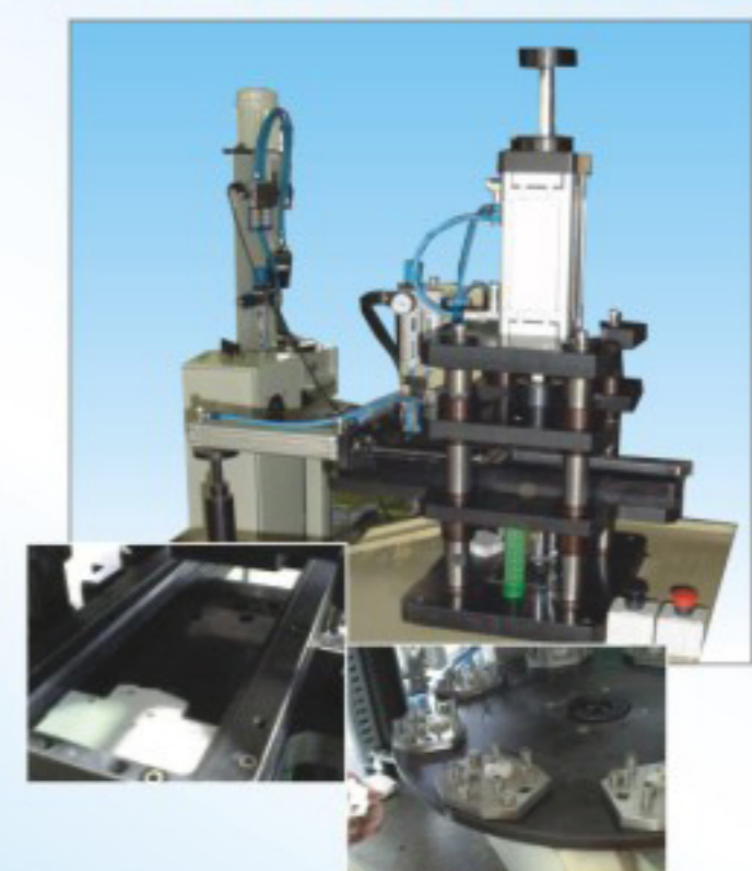
Modular Riveting SPM for MCB
