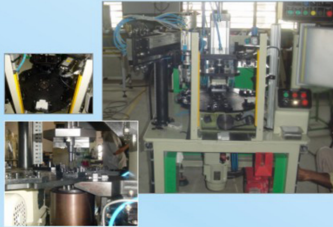
Multi Point Modular Riveting SPM for MCB
