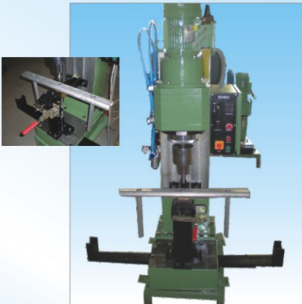
Riveting Machine for Aluminum Staircase
