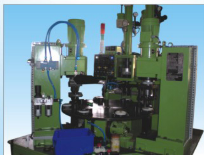
Flaring, Pressing & Trimming machine for Brush Assembly
