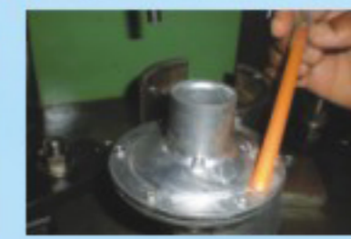
Retention Plate Riveting Machine for Door Latch Assly
